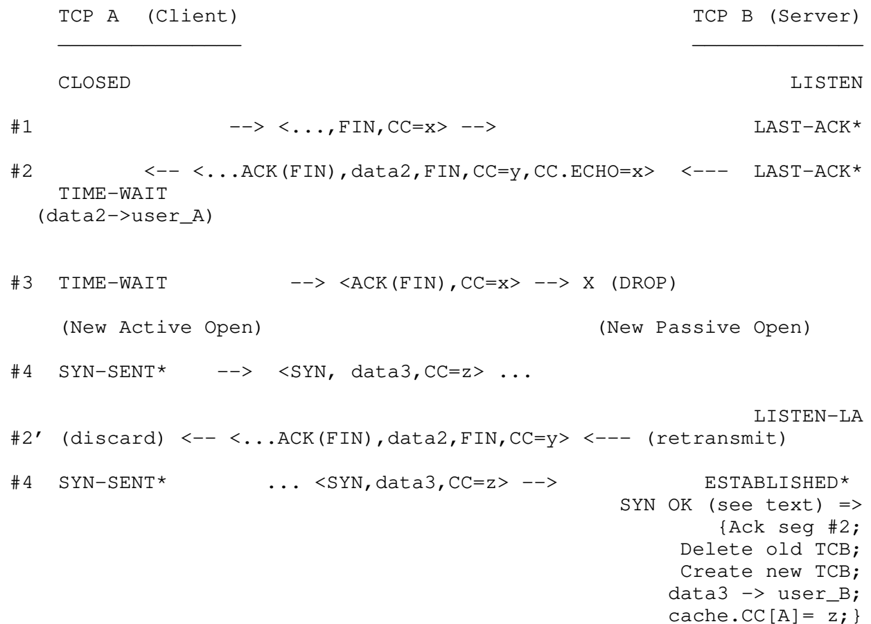
Figure 5: Truncating TIME-WAIT State: SYN as Implicit ACK
