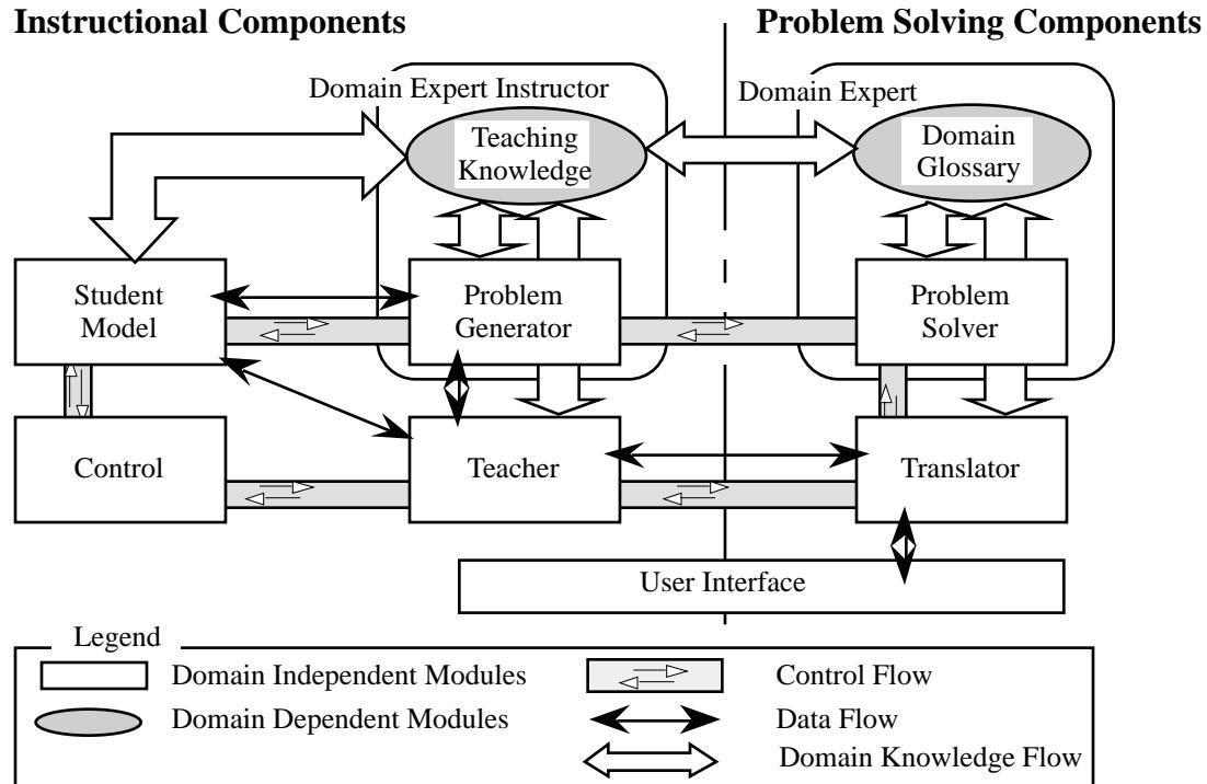
**Figure 1.** System architecture of I<sup>3</sup>'s intelligent teaching system
