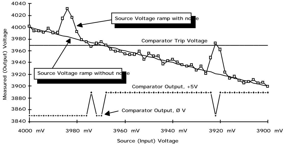
**Figure 3.** Noise Waveform During Test
