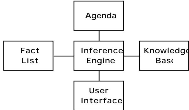
**Figure 4.** CLIPS Basic Components. Adapted from [6].
