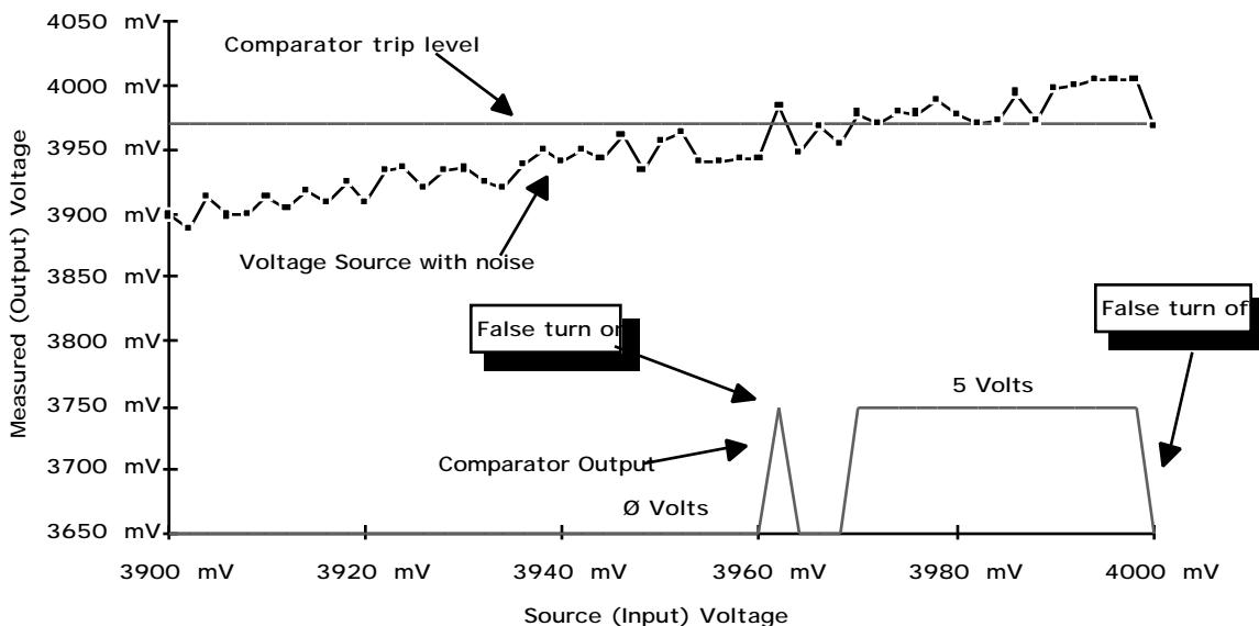
**Figure 2.** Comparator Output With a Noisy Source Signal
