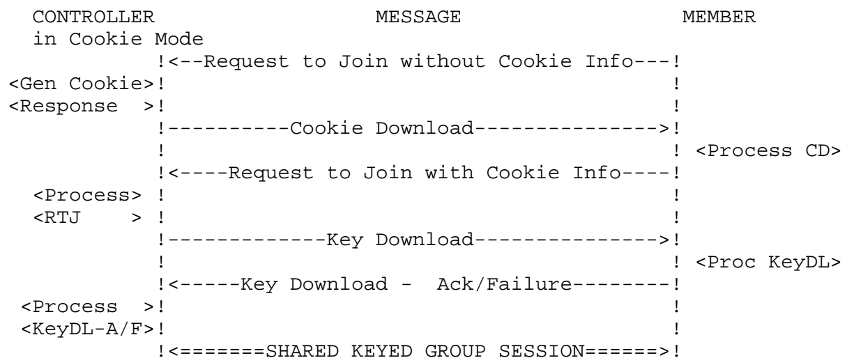
Figure 2: GSAKMP Ladder Diagram with Cookies
